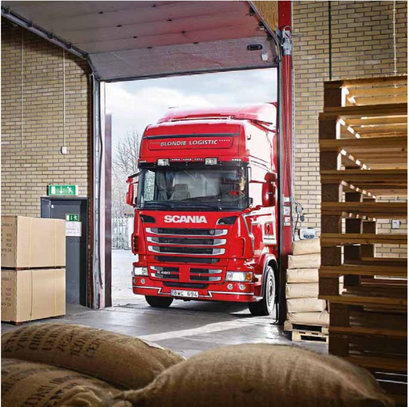
ECO-FIT – The trucks are fitted with reduced rolling resistance tires, while large air deflectors on the roof of the tractor unit help to reduce air resistance.
